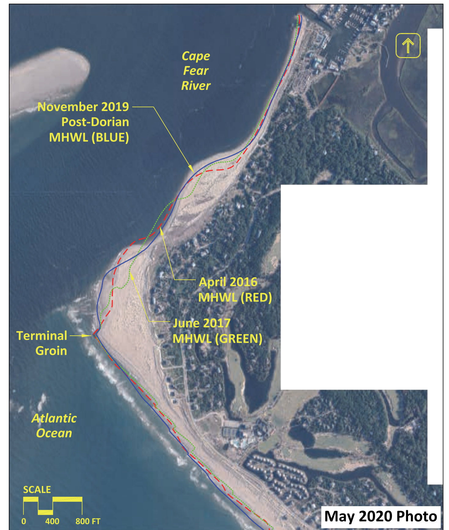
Figure 3.8: MHWL positions in the vicinity of the terminal groin Bald Head Island, NC
