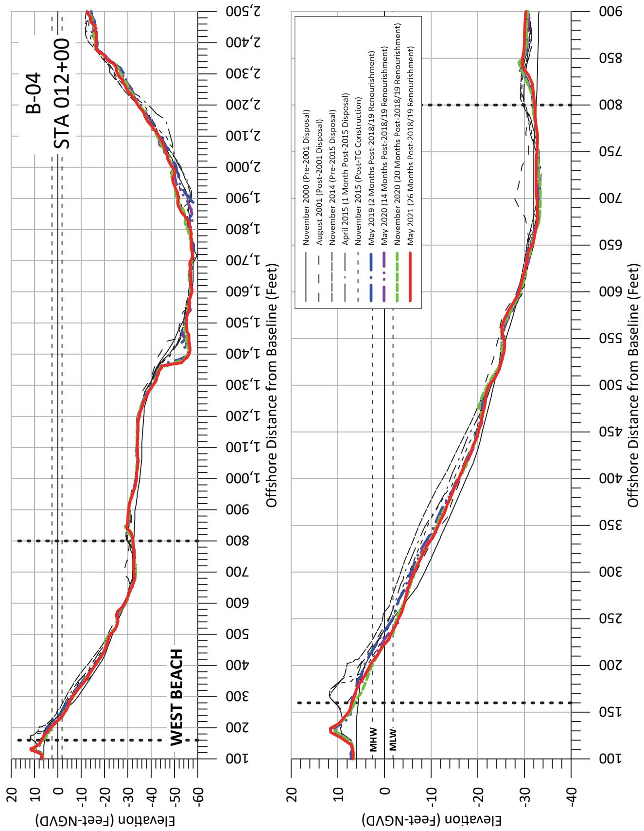
**Figure A-10:** Measured beach profiles at baseline **Station 012+00**, Bald Head Island, N.C.
