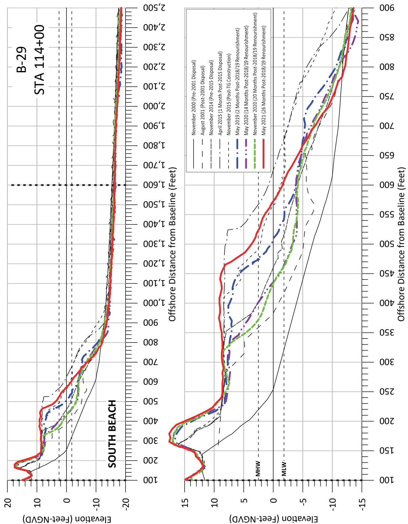
**Figure A-46:** Measured beach profiles at baseline **Station 114+00**, Bald Head Island, N.C.
