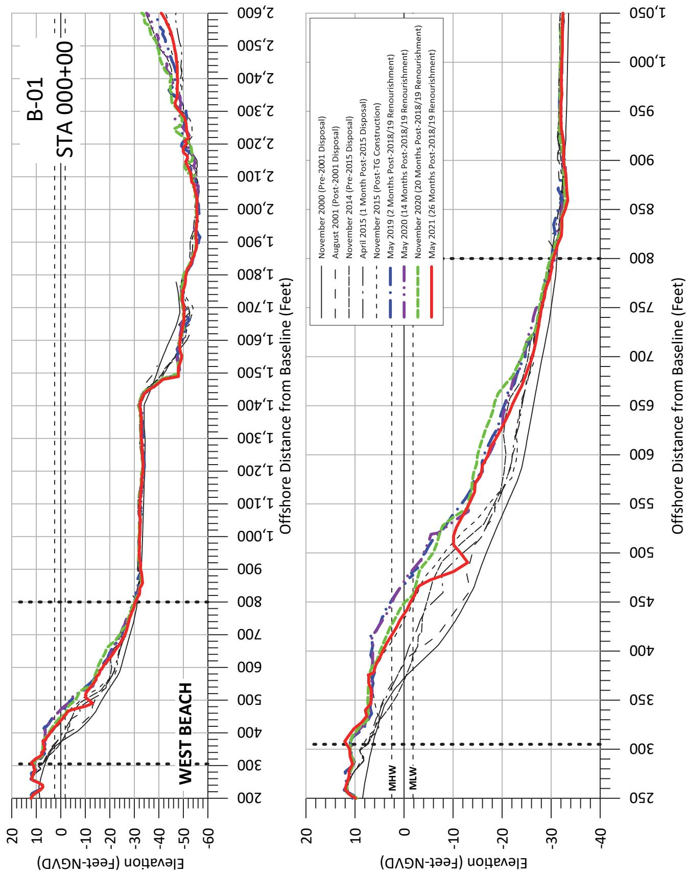
**Figure A-06:** Measured beach profiles at baseline **Station 000+00**, Bald Head Island, N.C.
