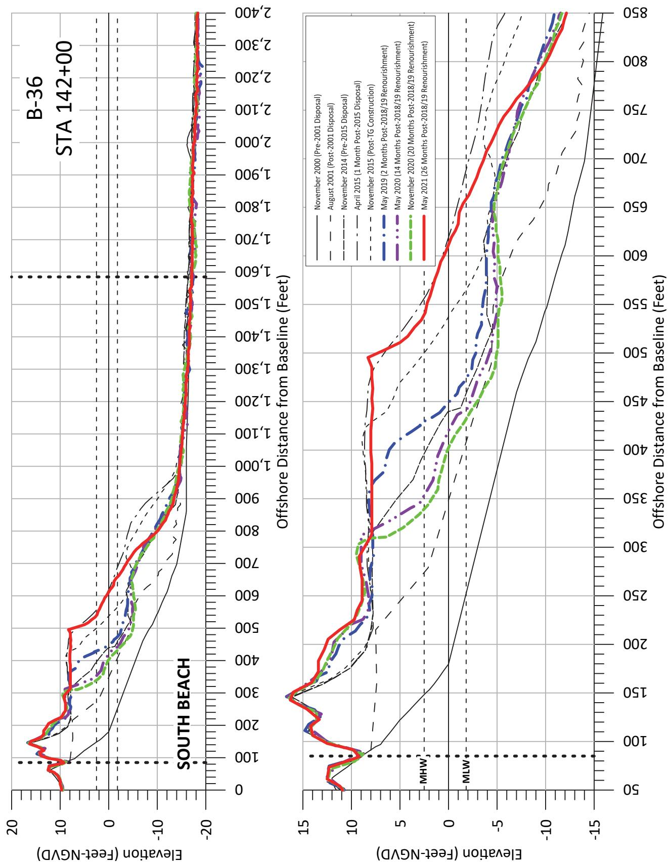
**Figure A-53:** Measured beach profiles at baseline **Station 142+00**, Bald Head Island, N.C.
