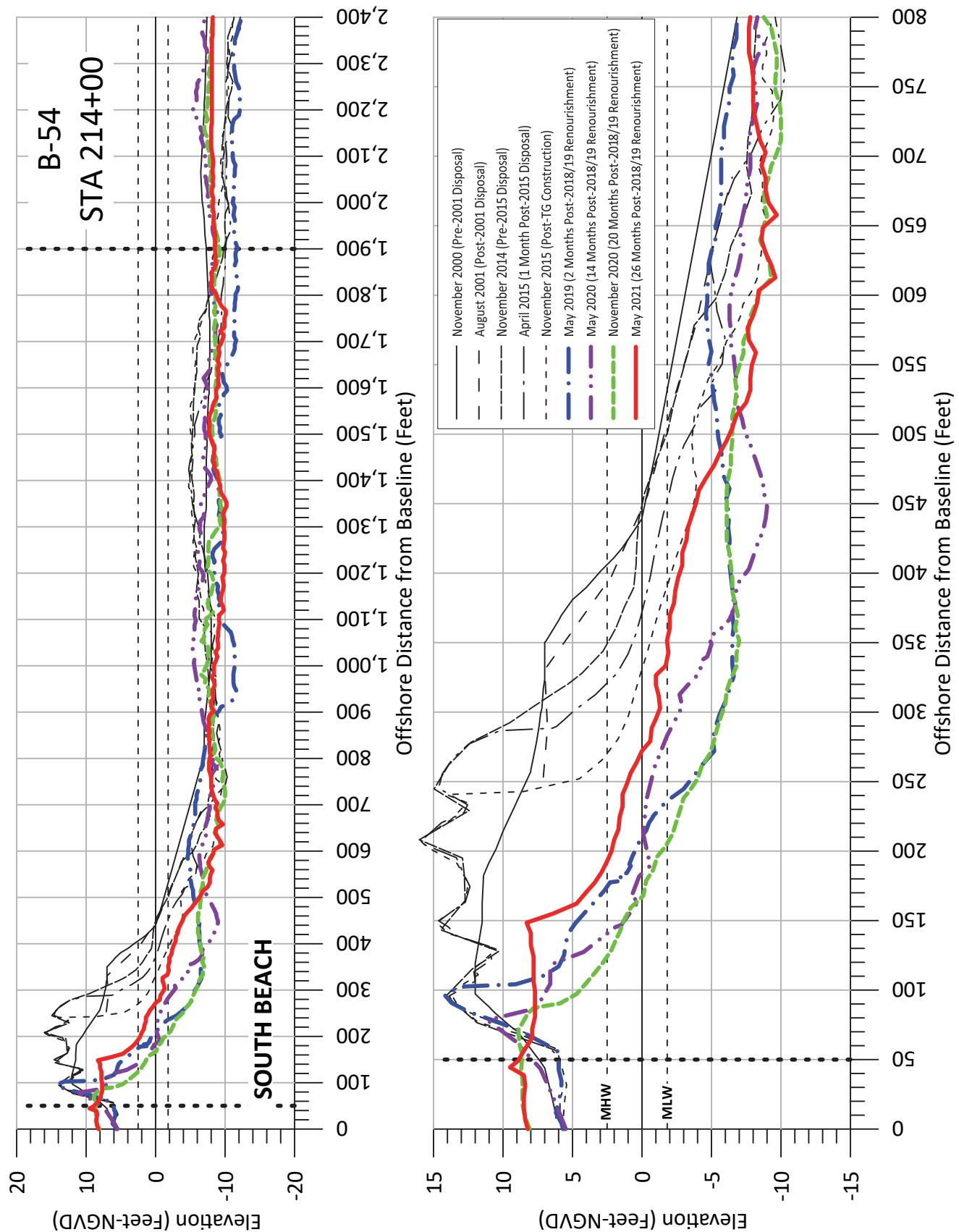
**Figure A-71:** Measured beach profiles at baseline **Station 214+00**, Bald Head Island, N.C.
