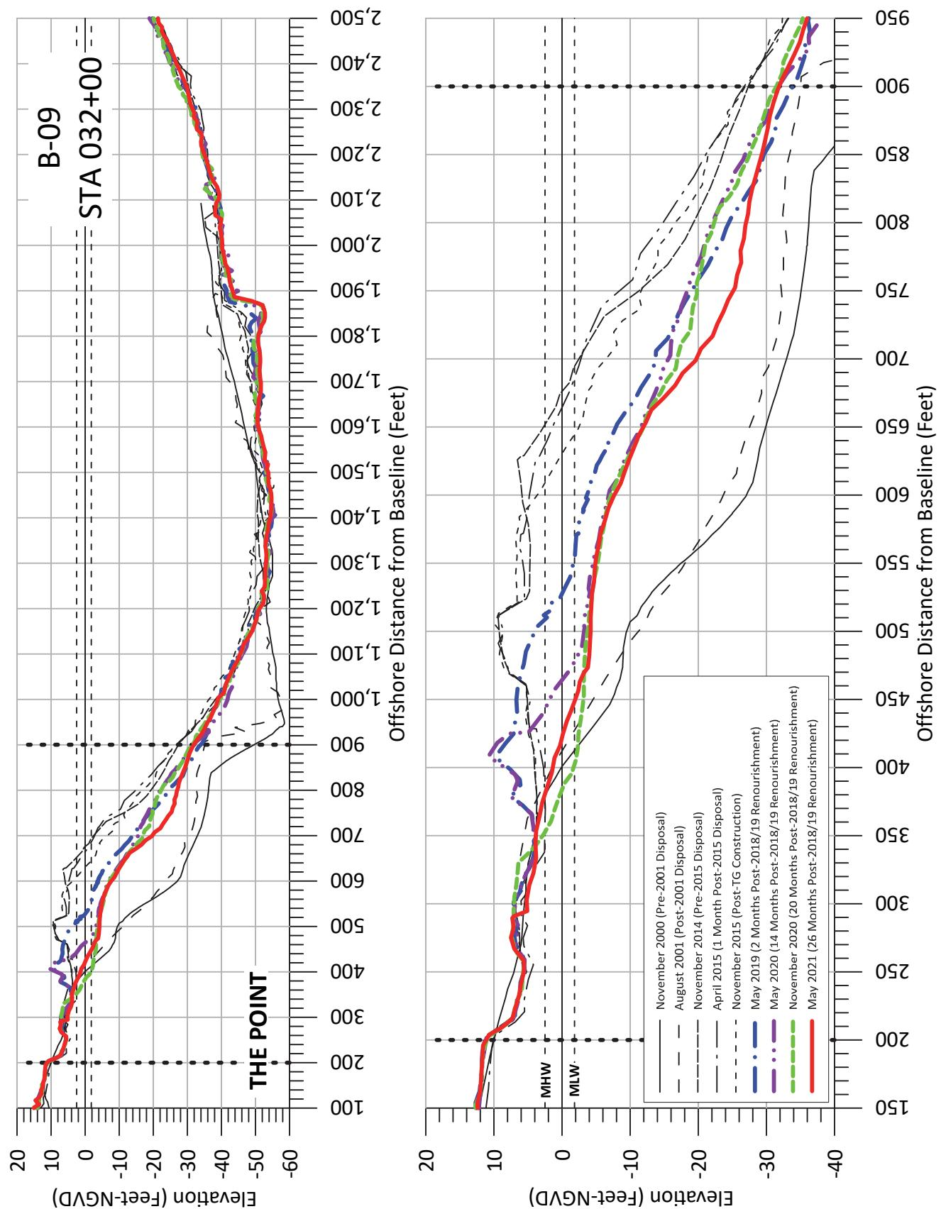
**Figure A-17:** Measured beach profiles at baseline **Station 032+00**, Bald Head Island, N.C.
