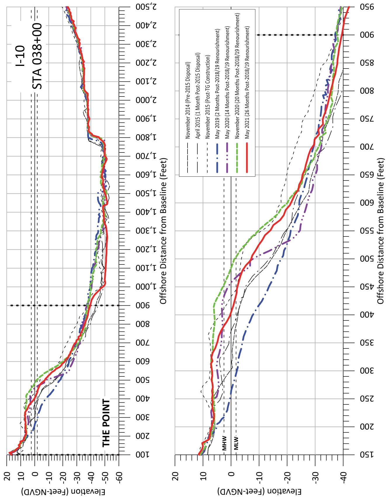
**Figure A-20:** Measured beach profiles at baseline **Station 038+00**, Bald Head Island, N.C.
