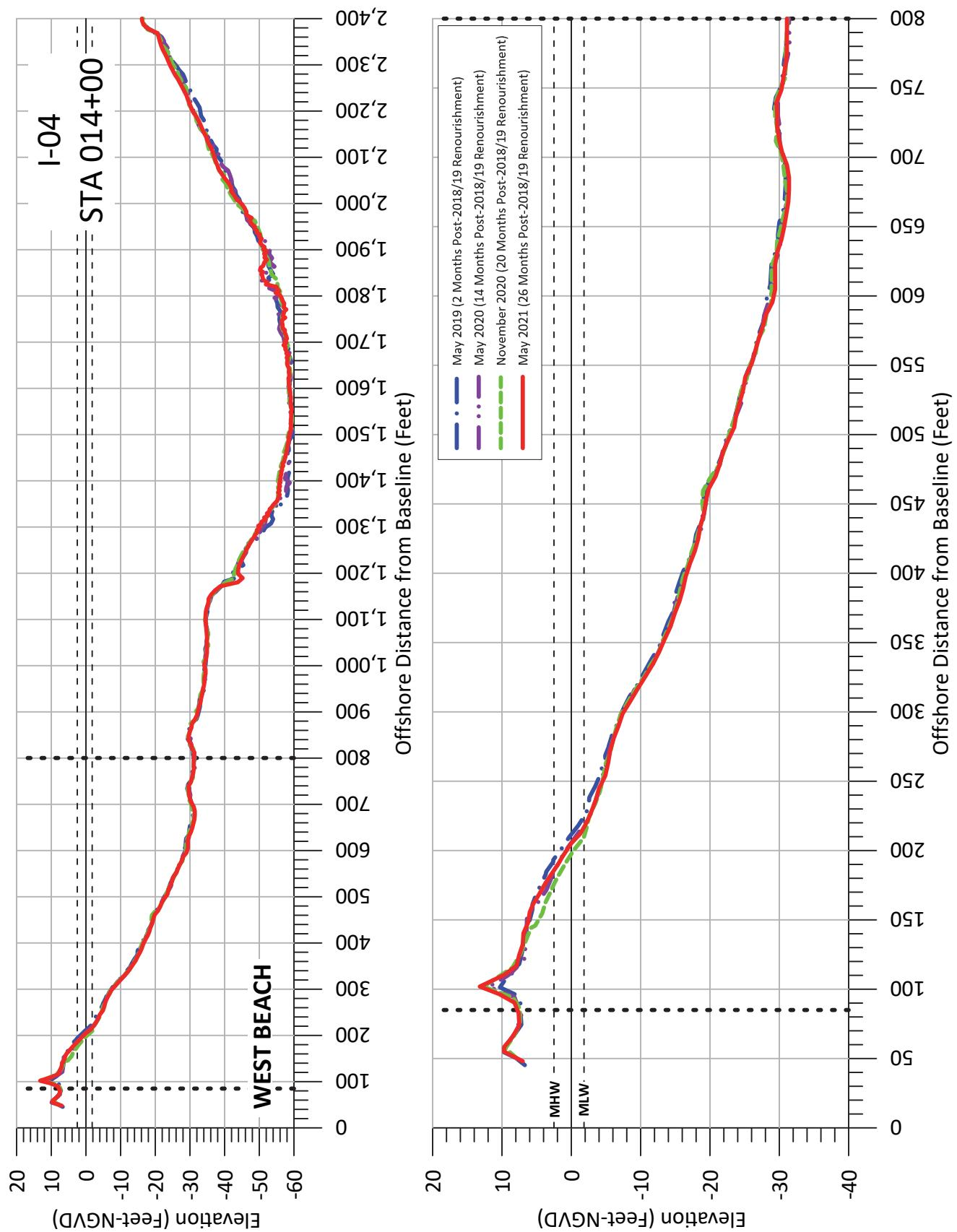
**Figure A-11:** Measured beach profiles at baseline **Station 014+00**, Bald Head Island, N.C.
