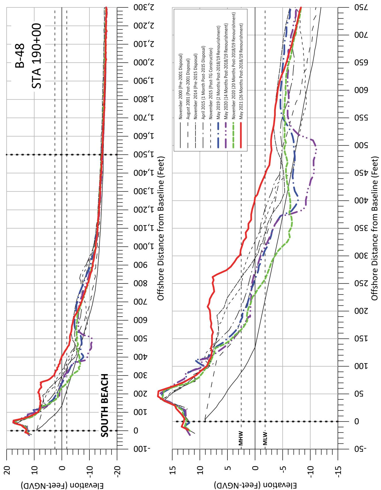
**Figure A-65:** Measured beach profiles at baseline **Station 190+00**, Bald Head Island, N.C.
