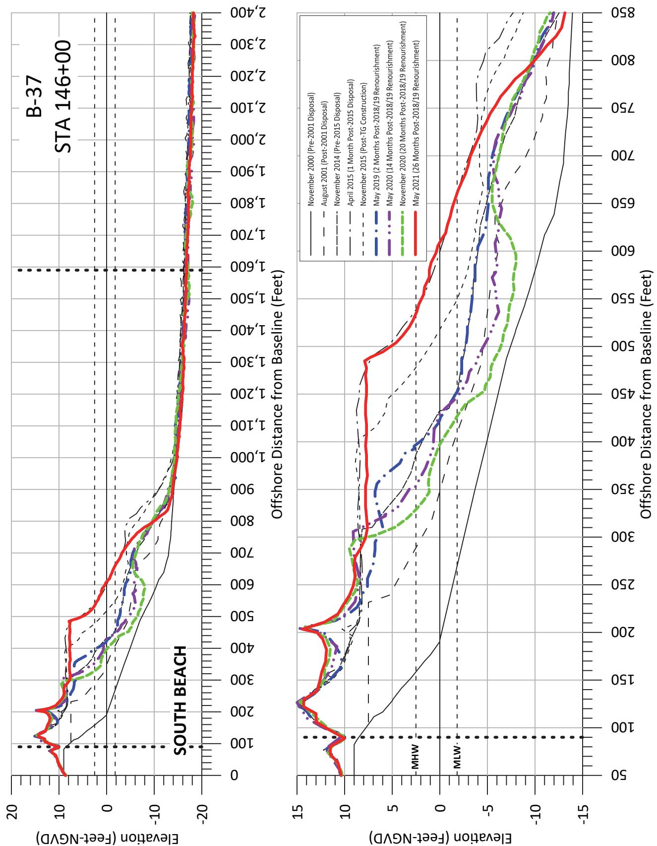
**Figure A-54:** Measured beach profiles at baseline **Station 146+00**, Bald Head Island, N.C.
