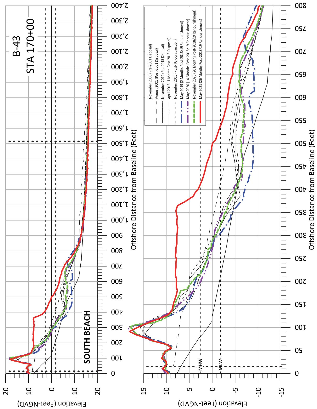
**Figure A-60:** Measured beach profiles at baseline **Station 170+00**, Bald Head Island, N.C.
