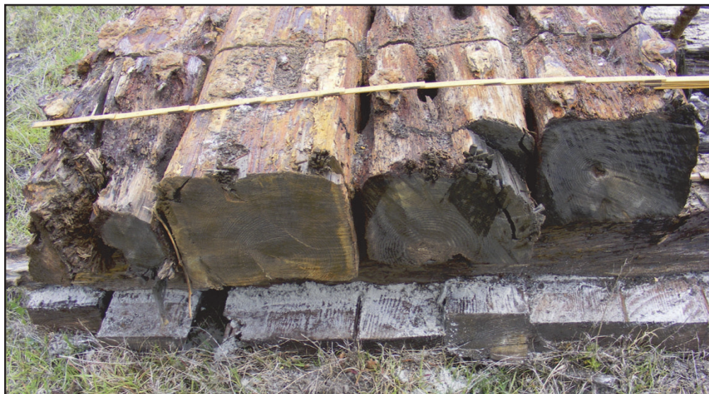
Figure 11. Shelf clamp timbers and futtocks with attached hull planking.
