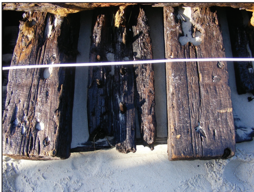
Figure 6. Futtock dimensions and space.
