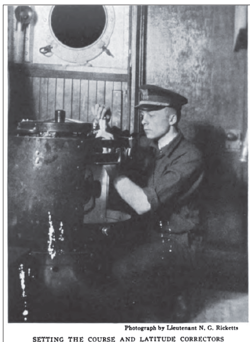
Figure 37. 1926 view of Modoc's state-of-the art gyro compass (Presented in: Zeusler 1926:22).
