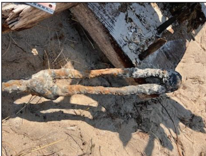
Figure 21. Turnbuckle attached to the eye stub.
