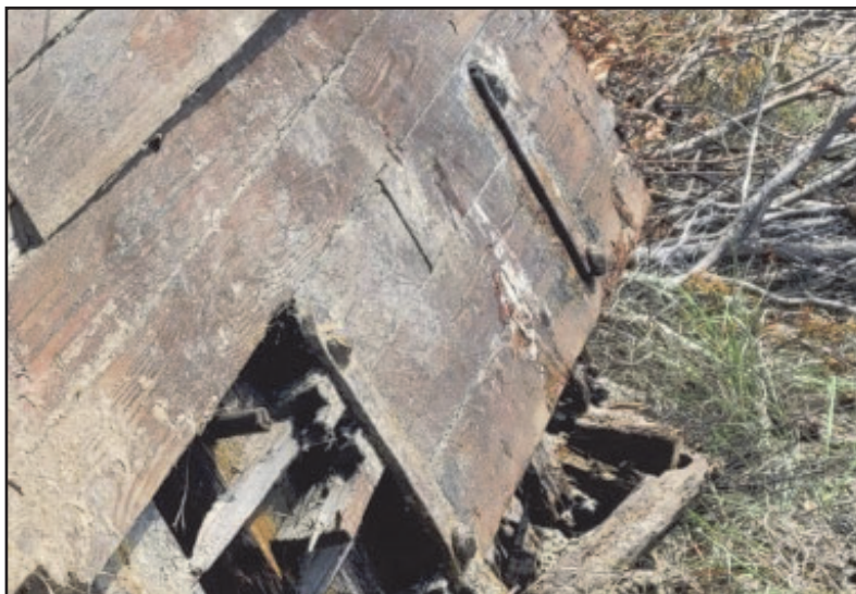
Figure 19. Iron straps attached the standing rigging turnbuckles to the hull.
