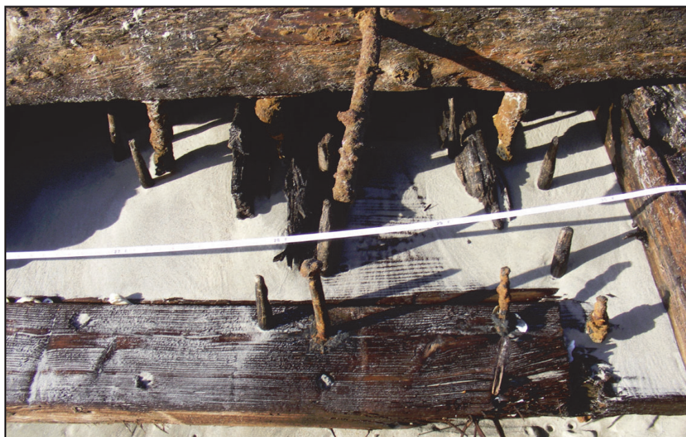
Figure 12. Hull plank with iron bolt, spike, and trunnel fasteners.
