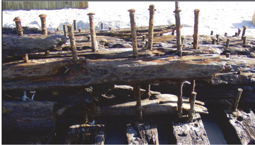
Figure 16. Top outboard shelf clamp timbers with diagonal scarf.
