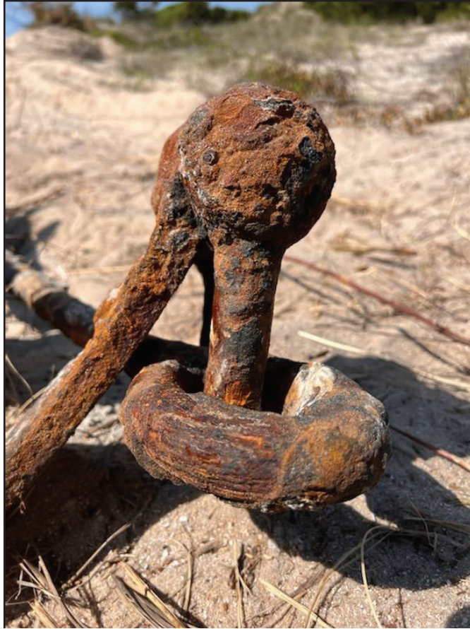
Figure 20. Shackle connected to the hull strap with the turnbuckle stub eye attached.
