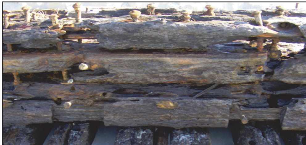
Figure 18. Top timber in the shelf clamp with rebates for deck beams.
