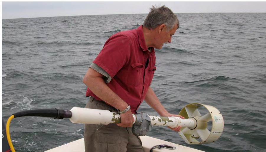
Figure 3. Launching the Geometrics 881 Cesium Vapor magnetometer.
