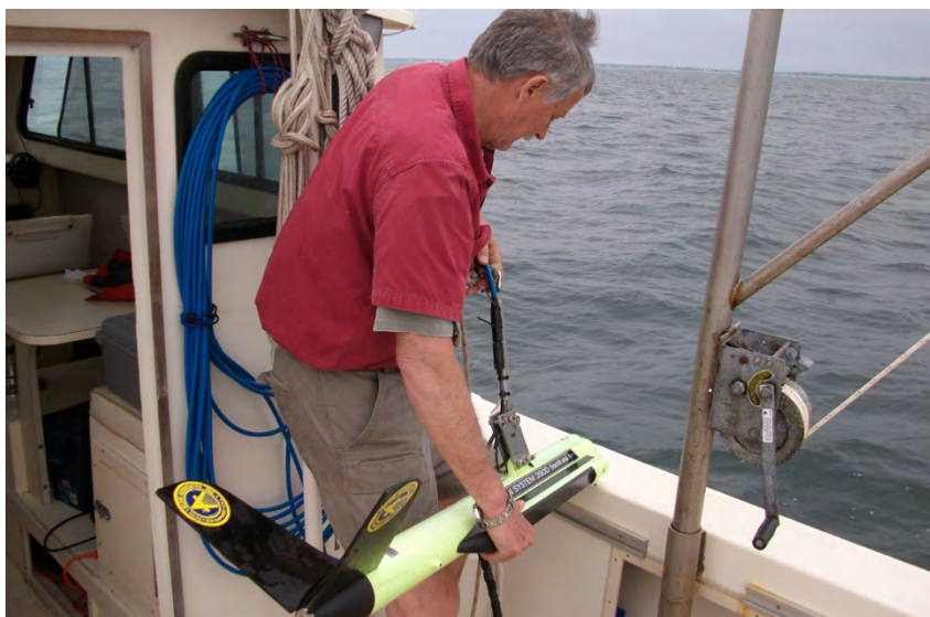
Figure 4. Launching the Klein 3900 sidescan sonar.
