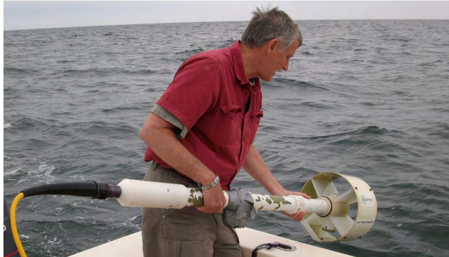
Figure 3. Launching the Geometrics 881 Cesium Vapor magnetometer.
