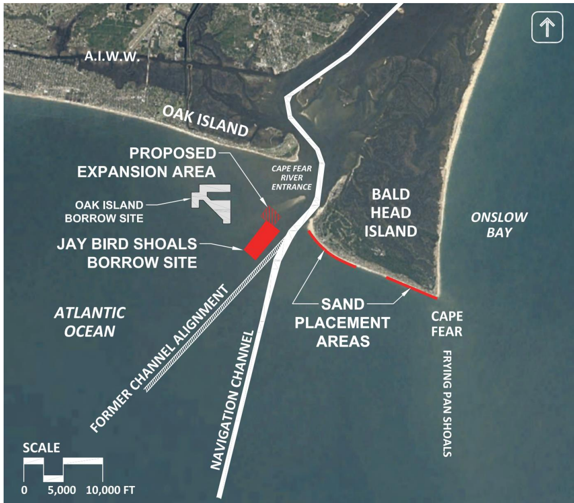
Borrow site and sand placement areas for the 2025 CDSR Project (Photo from Project Plans submitted to USACE)
