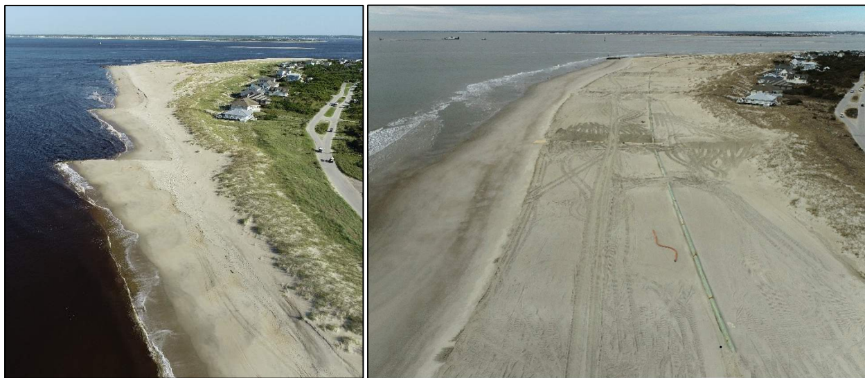
Photograph 1.1: Pre-(August 2024) and post-beach fill placement (January 2025) at the western limit of the project, just east of the terminal groin. Note that the sand-tube groins are buried in the post placement photograph.
